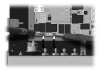
Remove plastic cover and measure voltage between two heater screws on the board.
