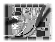
3 • Verify if you can get a reading of I 20 VAC for fiber box motor and light output.
