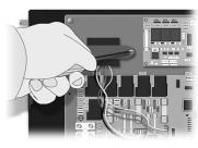
4• If GFCI still trips, replace transformer. If it stops tripping, reconnect one component at a time until GFCI starts to trip. Replace defective component. If GFCI continues to trip even after having replaced the transformer, carry out the following tests to correct the problem:
