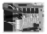
Turn Pump I to low speed and measure voltage between white and red wire connectors: 240 VAC pump: P37 & P57 I 20 VAC pump: P37 & P48
