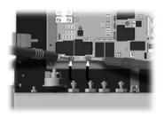
3 • Remove spa cover. With a voltmeter, read the voltage between the two heater wires on the board. 4• If you do not read 240 VAC, pump may be overheating water during filter cycle.
