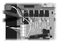
3 • Turn Pump I to high speed and measure voltage between white and black wire connectors: 240 VAC pump: P64 & P57 I 20 VAC pump: P64 & P48
