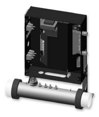
5 • Slide new heater into place and attach it to the enclosure using the two nuts.
