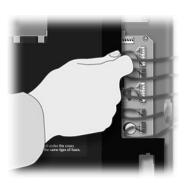
2. Unplug keypad(s) and all connectors located on the right side of the power box.
