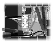
3 • Measure voltage between ozonator white and black wire connectors: 240 VAC ozonator: P30 & P60 120 VAC ozonator: P30 & P46
