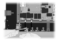
2. If voltage reading is correct, verify if heater wires are properly connected to the element.
