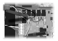
3 • Turn Pump 2 to high speed and measure voltage between white and black wire connectors: 240 VAC pump: P35 & P58 120 VAC pump: P35 & P45
