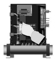
4 • Lift up the cover starting on the left side and slide it out from the guide points.
