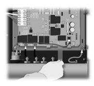
6• Unscrew wing nut that holds hilimit latch in place. Slide out hillimit sensor.
