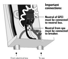
2 • If it is not, verify GFCI wiring diagram and reconnect it.
