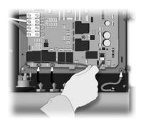
5• Disconnect pressure switch cable and light socket.
