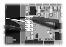
On the terminal block, measure voltage between line 1 and line 2.
