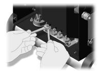
2. With wrenches, disconnect heater by removing the fours nuts on top of the elements.
