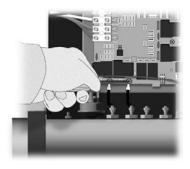
7 • Disconnect heater output by removing 3 screws at the bottom of circuit board on heater.
