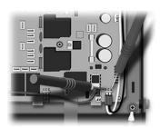
3 • Remove plastic cover and measure voltage between opposite prongs of connector P14 on the board.
