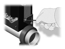
4 • Loosen the two screws that hold mounting feet on each side of the pack and slide heater out.
