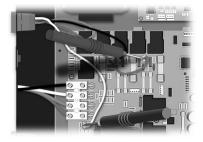
Turn pump 2 to low speed and measure voltage between white and red wire connectors: 240 VAC pump: P22 & P58 120 VAC pump: P22 & P45
