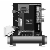
3 • Remove 2 screws that hold metal cover in place (on the left side of the power box).
