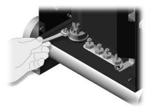
3 • Unscrew the two nuts that hold heater to the enclosure and slide heater from under the pack.
