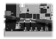
2 • If the water temperature is lower than the desired temperature, measure the voltage to the heater.
