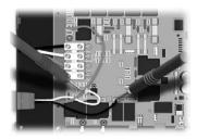
3 • Remove plastic cover and take voltage reading between circulation pump's black and white wire connectors.
