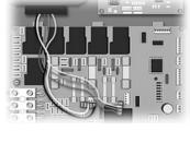
3 • If nothing works, clean transformer orange connector pins. Even a small coating of film may cause a bad connection.
